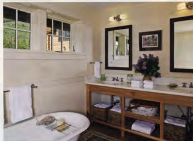
Awning windows set high on the north side of the house keep the master bath private and passively cooled.
